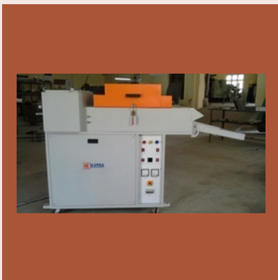
Nano Roller Coater with UV+IR
