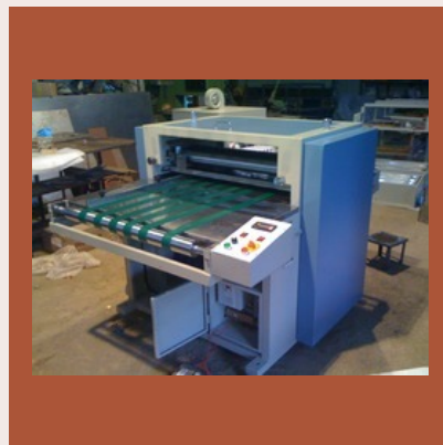
UV Varnish Roller Coater
