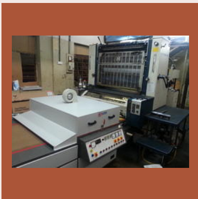
UV Attachment To Offset Press
